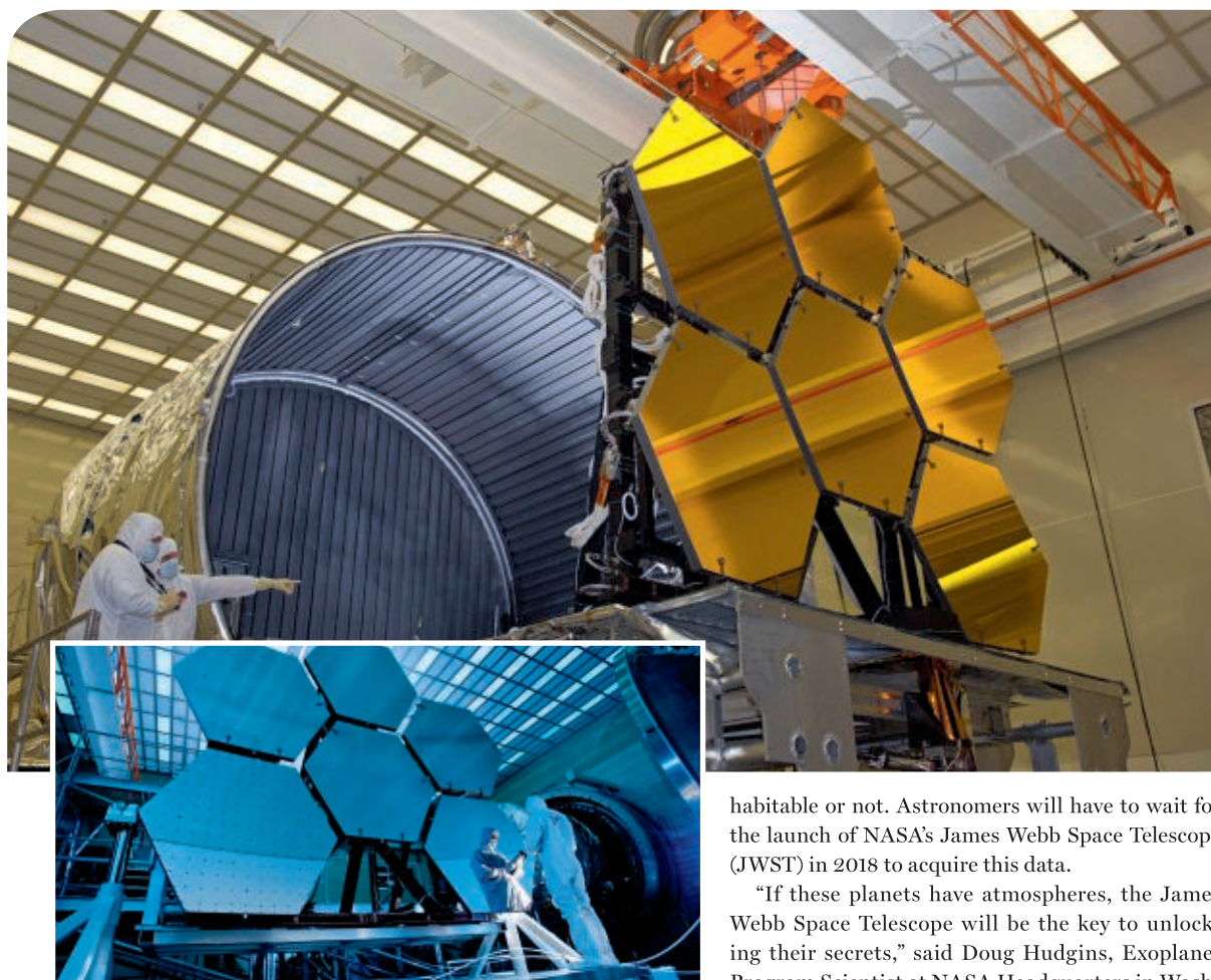
Top and above: The James Webb Space Telescope will have 18 large mirrors when completed, enabling it to analyze the atmospheres of exoplanets.
